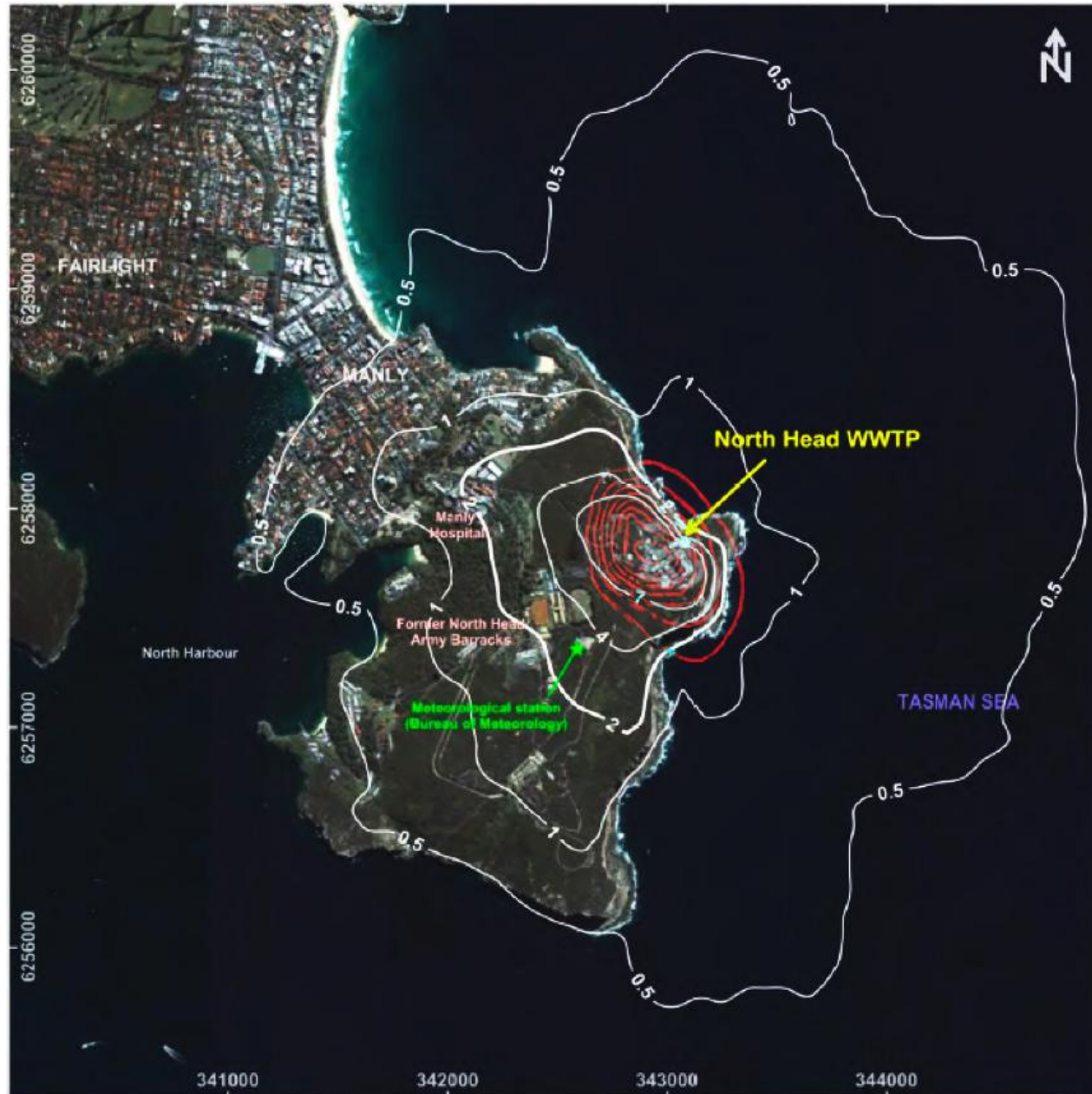
Map 2 – Malabar proposed Final Odour Contours Superimposed on North Head Proposed Final Odour Contours
